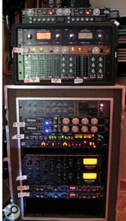
This rather fuzzy photo shows the labels illustrating how some of the other outboard gear was assigned. Visible from top are Empirical Labs EL7 Fatso tape simulator, SSL compressor, a pair of Universal Audio LA3A compressors, another EL7, a rack of API EQs, Neve 33609 compressor, a pair of Empirical Labs Distressor compressors, API 2500 compressor, Eventide 2016 reverb, Slate Dragon compressors (x2) and Lexicon PCM42 delay (x2).
