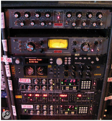
Adding his own gear to that resident at 5150 gave Ross Hogarth a powerful mixing arsenal. In this rack, from top, are a Retro Instruments 2A3 EQ and 176 compressor, Bricasti M7 reverb, Chandler TG1 limiter, and two AMS DMX 15-80 delays with a TC Electronic 2290 delay between.
