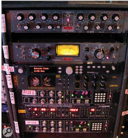
Adding his own gear to that resident at 5150 gave Ross Hogarth a powerful mixing arsenal. In this rack, from top, are a Retro Instruments 2A3 EQ and 176 compressor, Bricasti M7 reverb, Chandler TG1 limiter, and two AMS DMX 15-80 delays with a TC Electronic 2290 delay between.
